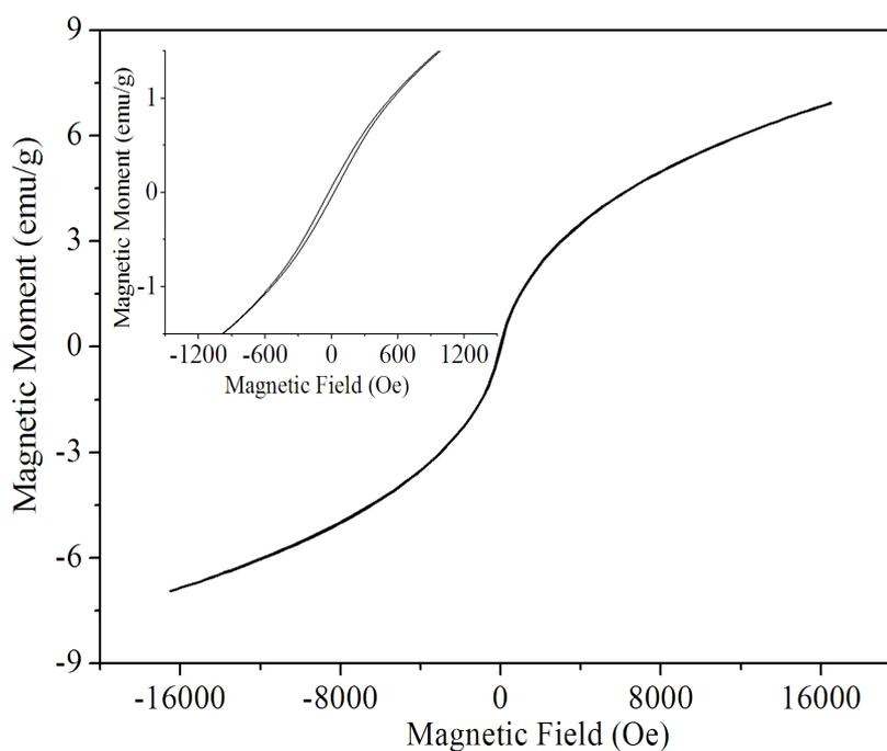
**Figure 7.3** Room temperature hysteresis curve obtained for  $Gd_2O_3/NiFe_2O_4$  CSNPs. The inset Figure shows the hysteresis plot for the lower values of the magnetic field.
