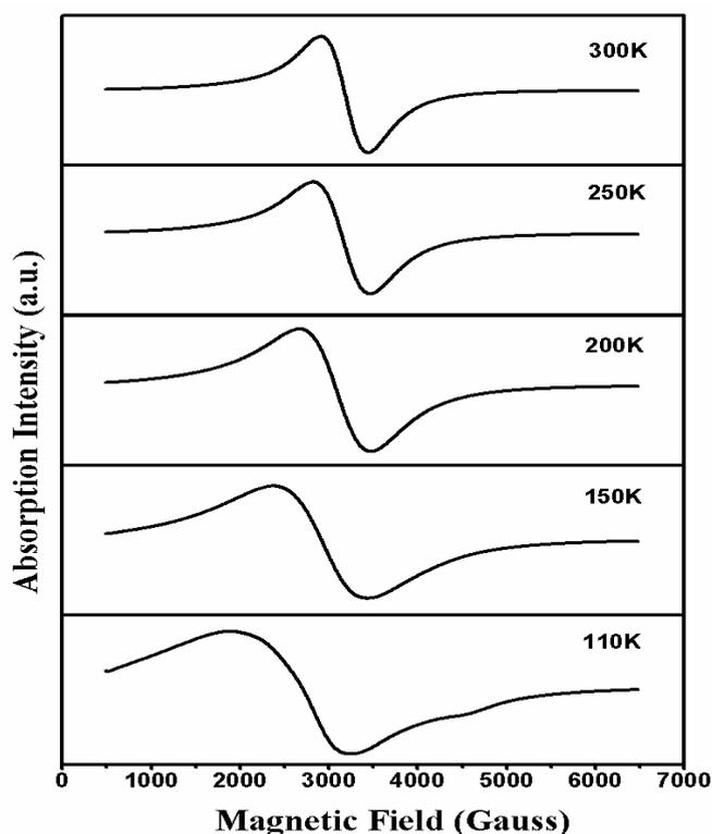
**Figure 7.4** EPR spectra obtained for  $\text{Gd}_2\text{O}_3/\text{NiFe}_2\text{O}_4$  CSNPs at low temperatures
