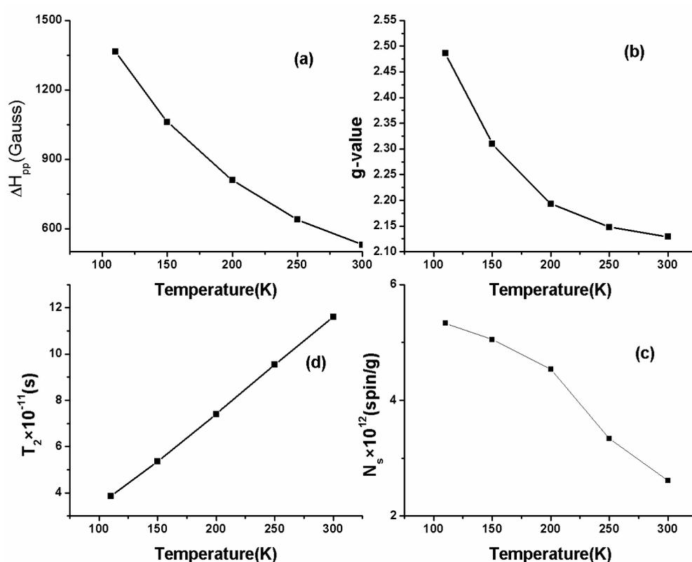
**Figure 7.5** Variation of (a) peak to peak line width ( $\Delta H_{pp}$ ) with temperature, (b) g-factor with temperature, (c) spin concentration ( $N_s$ ) with temperature and (d) relaxation time ( $T_2$ ) with temperature for  $Gd_2O_3/NiFe_2O_4$  CSNPs
