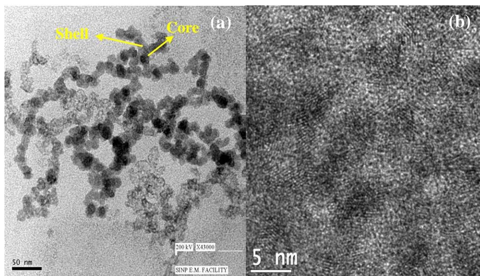
**Figure 7.2** (a) TEM micrograph obtained for  $Gd_2O_3/NiFe_2O_4$  CSNPs (b) HRTEM micrograph obtained for  $Gd_2O_3$  core
