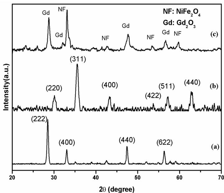
**Figure 7.1** X-ray diffraction patterns of (a)  $Gd_2O_3$ , (b)  $NiFe_2O_4$  and (c)  $Gd_2O_3/NiFe_2O_4$  NPs
