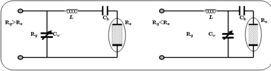
Figure 2.3 Impedance matching networks for RF-sputtering system
