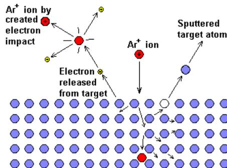
Figure 2.1 Incident ions and the sputtered particles [105]
