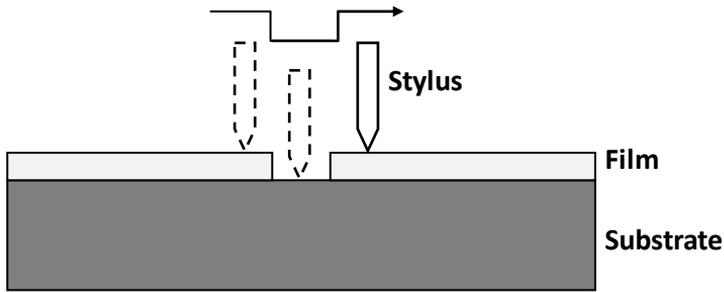
Figure 2.7 Illustration of stylus profilometer measure film thickness
