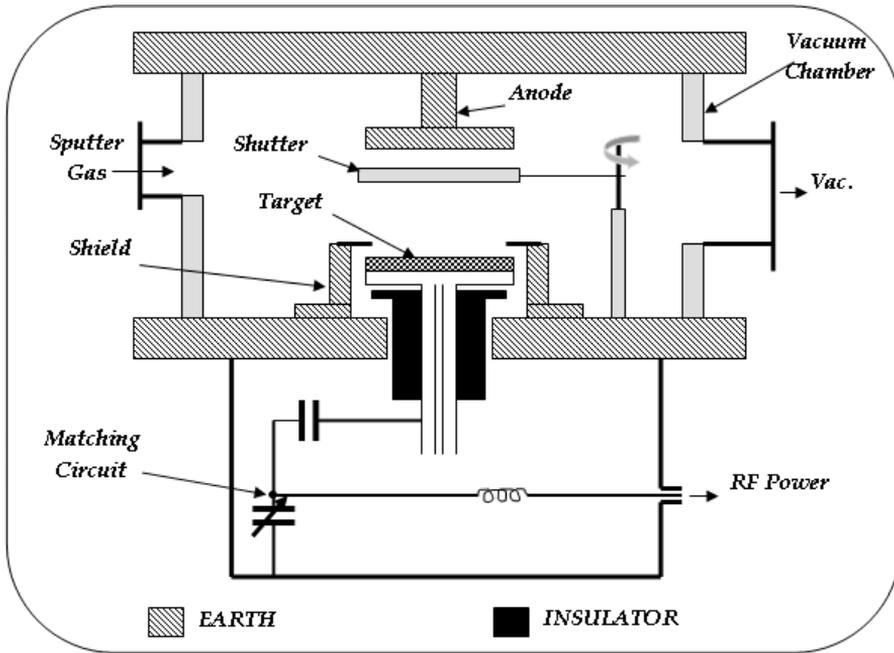
Figure 2.2 schematic view of an RF magnetron sputtering
