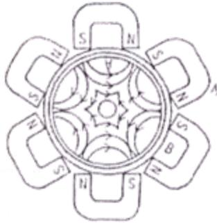
Figure 2.4 Cross-sectional view of the planar magnetron sputtering
