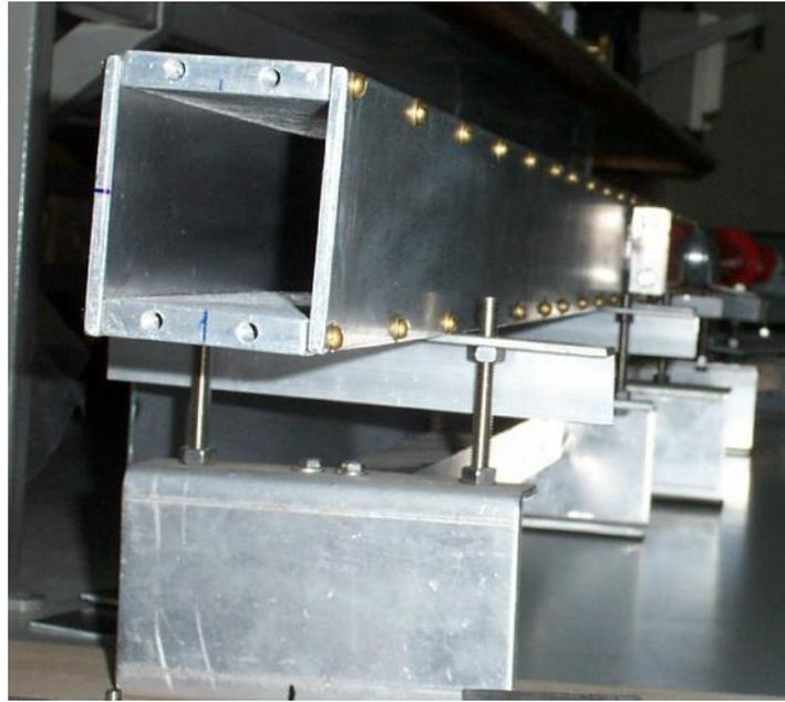
Figure 4.5 Square corrugated waveguide
