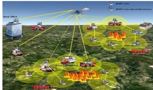
salvage operations should take place where there is no accessible infrastructure or broken infrastructure and in such an environment quick deployment of a communication network is required. Information is forwarded using small hand held portable devices from the member of one rescue team to another. MANETs can also be used with commercial scenarios like law enforcement, ship to ship ad hoc mobile communication etc.
