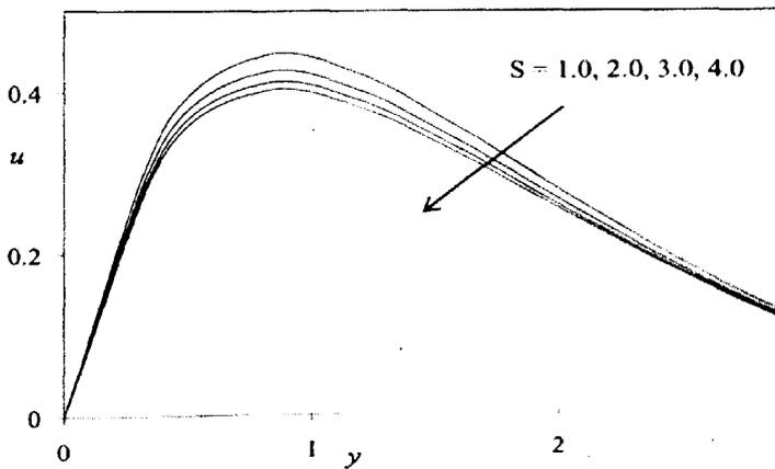
Figure 9. Velocity profiles for different values of  $S$
