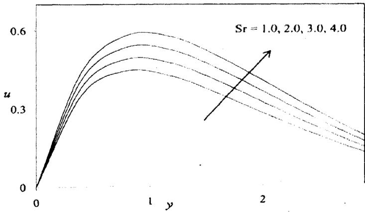
Figure 11. Velocity profiles for different values of  $Sr$
