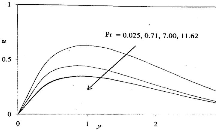
Figure 4. Velocity profiles for different values of  $Pr$
