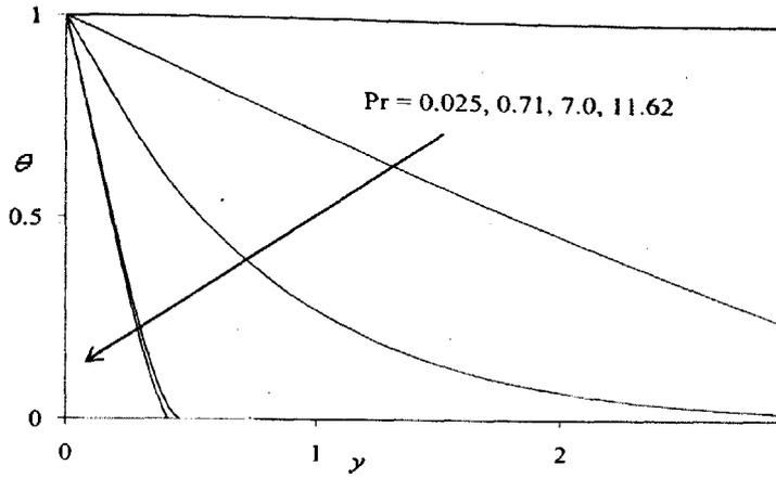
Figure 12. Temperature profiles for different values of  $Pr$
