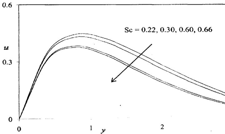
Figure 5. Velocity profiles for different values of  $Sc$
