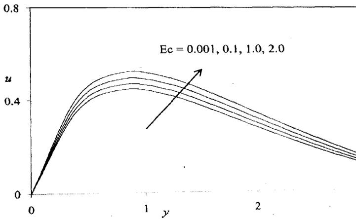
Figure 7. Velocity profiles for different values of  $Ec$
