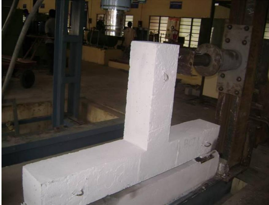
Fig. 3.20 Typical View of Beam-Column Joint Specimen
