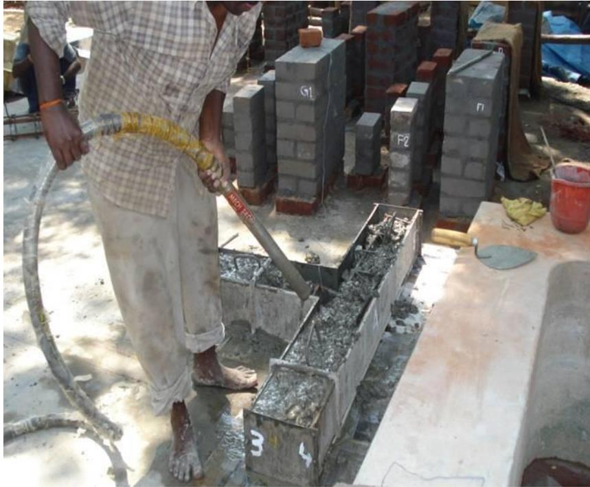
Fig.3.18 Typical View of Casting of Beam-Column Joint Specimen
