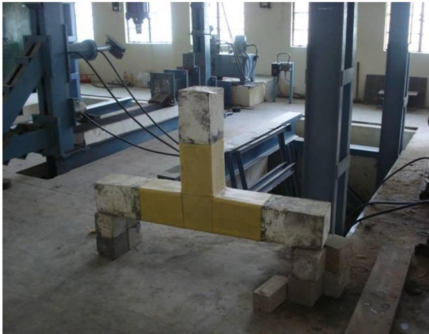
Fig.3.23 Typical View of Beam-Column Joint Specimen Retrofitted with AFRP Sheet
