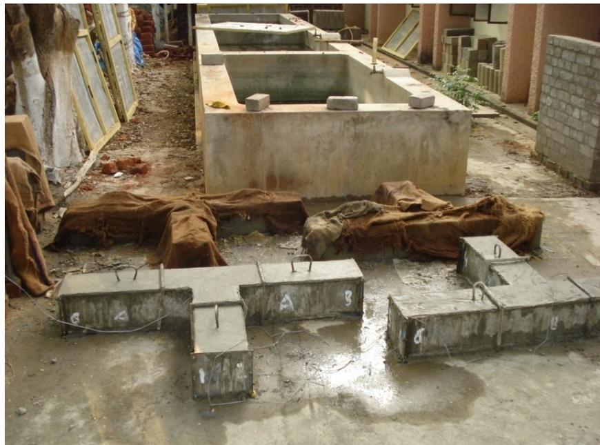
Fig.3.19 Typical View of Curing of Specimen
