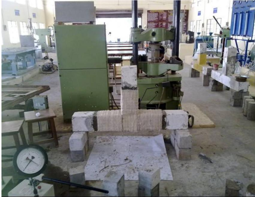
Fig.3.24 Typical View of Beam-Column Joint Specimen Retrofitted with Sisal Fiber Sheet
