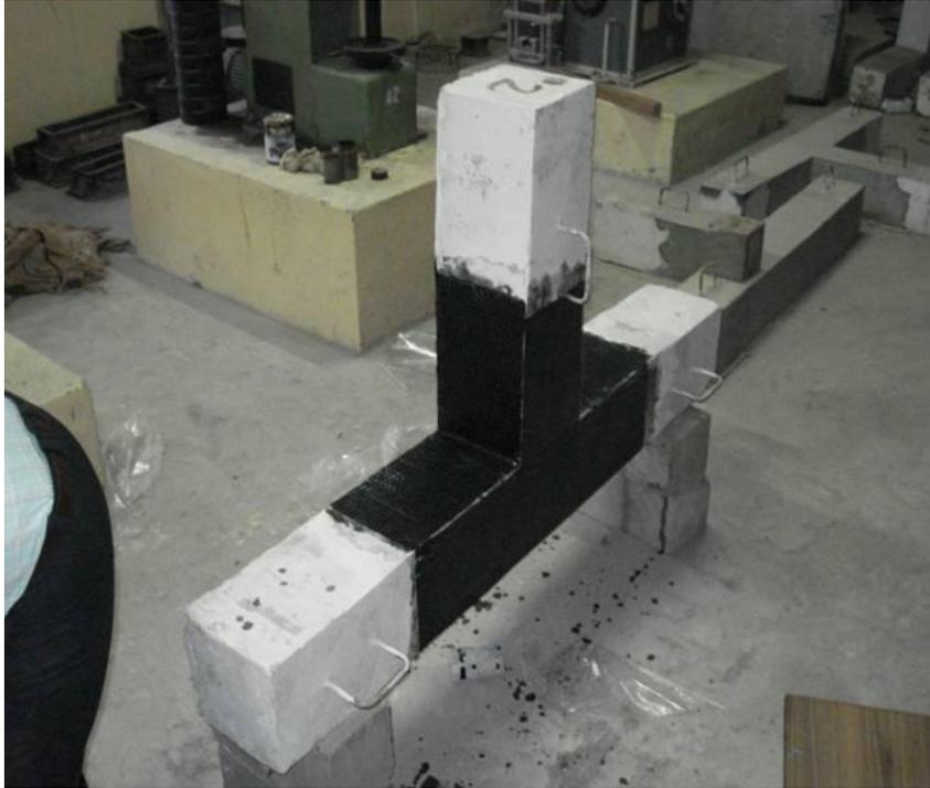
Fig.3.22 Typical View of Beam-Column Joint Specimen Retrofitted with CFRP Sheet
