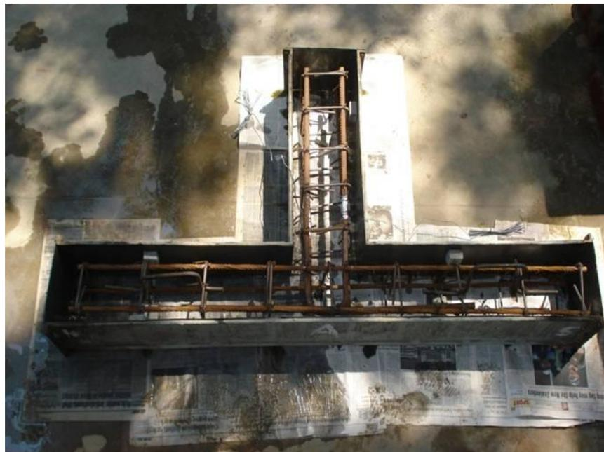
Fig.3.17 Typical View of Placing of Reinforcement in the Mould
