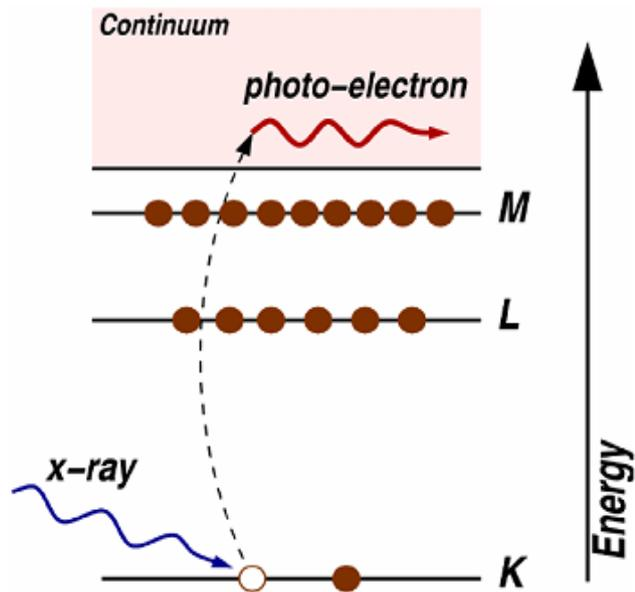
Fig. 2.2: Physics of X-ray Absorption (Newville, 2004)
