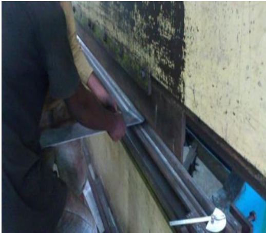
(a) Folding of Web Plate by Press-Break
