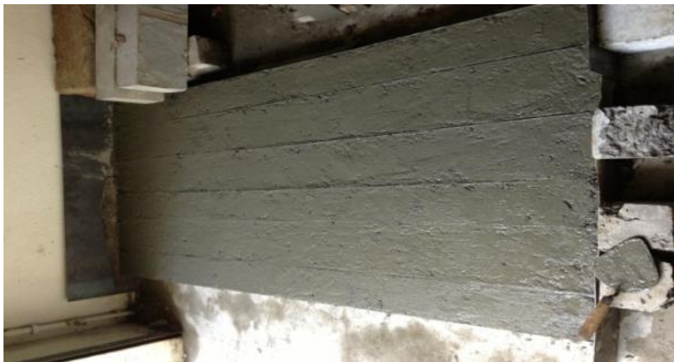
Figure 3.8 Specimens with Concrete Encased Web
