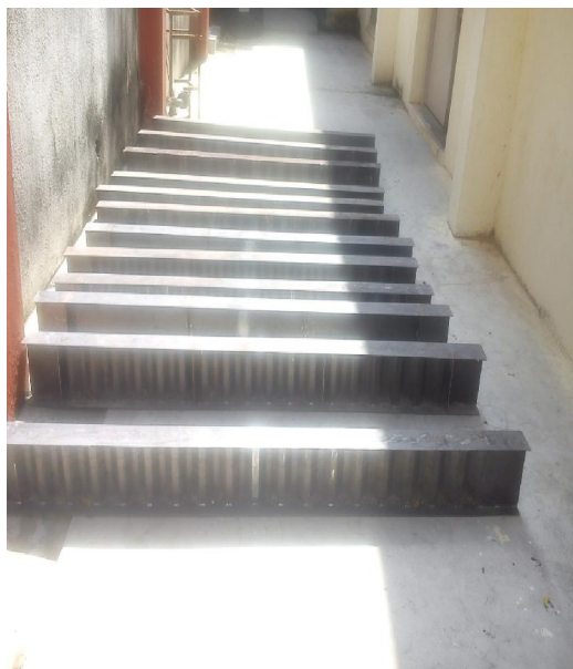
(a) Fabricated Specimens with Plain Web, 30 0 and 45 0 Corrugated Web Beam
