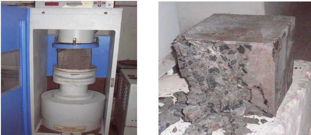
Figure 3.2 Experimental Set- up for Compression Strength.
