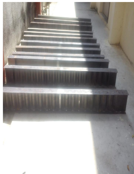
(a) Fabricated Specimens with Plain Web, 30 0 and 45 0 Corrugated Web Beam
