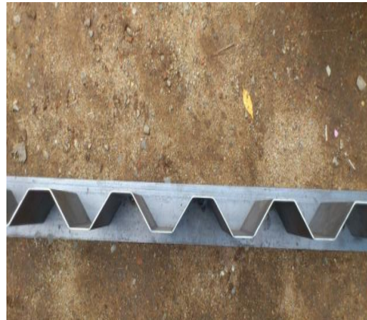
(d) View of the Corrugated Web Welded with the Bottom Flange
