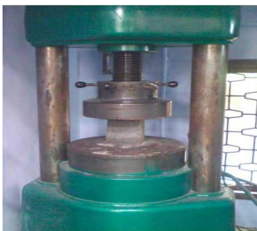
Figure A1.1 Compression testing of cube
