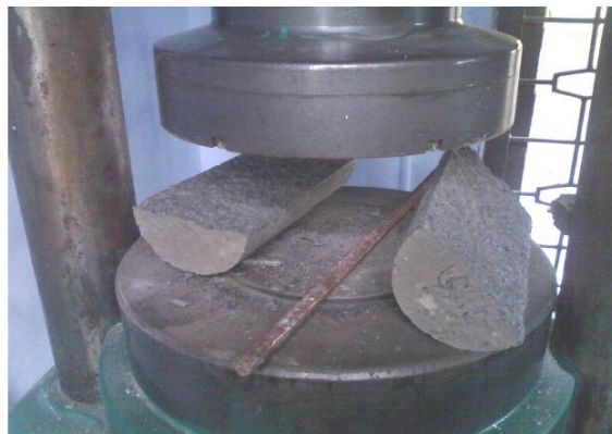
Figure A1.2 Split tension test for cylinder
