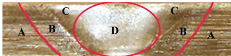
(A = Unaffected Base Metal; B = Heat Affected Zone (HAZ); C = Thermo-Mechanically Affected Zone (TMAZ); D = Friction Stir Processed (FSP) zone)
