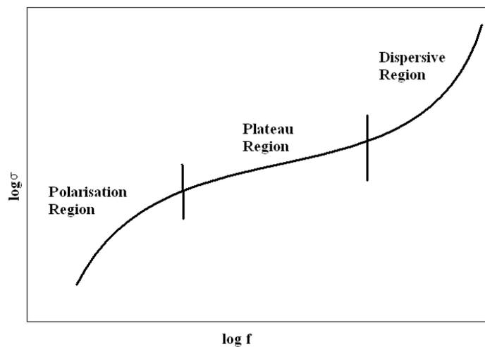
**Figure (3.21): schematic representation of log conductivity versus frequency**
