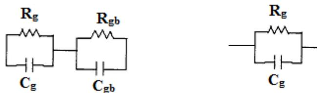
**Figure (3.14):** Equivalent circuit (a) for pure Pb levo-tartrate crystals (b) for mixed Pb-Fe levo-tartrate crystals
