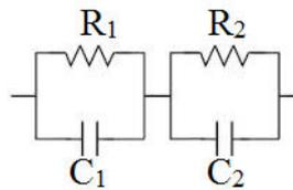
**Figure (3.11): Equivalent circuit, subscripts 1 and 2 refer to bulk and grain boundary components**
