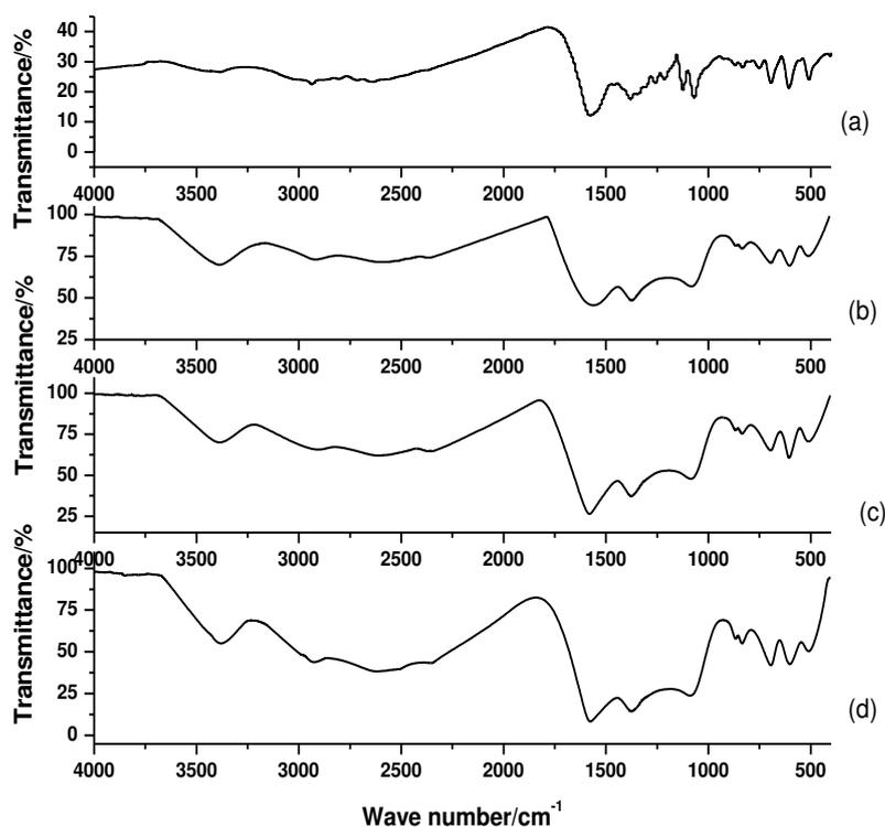
**Figure (3.7): FTIR spectra (a) Sample 1. Pure Pb levo-tartrate (b) Sample 3. Pb<sub>0.989</sub>Fe<sub>0.011</sub>C<sub>4</sub>H<sub>4</sub>O<sub>6</sub>·nH<sub>2</sub>O (c) Sample 4. Pb<sub>0.993</sub>Fe<sub>0.007</sub>C<sub>4</sub>H<sub>4</sub>O<sub>6</sub>·nH<sub>2</sub>O and (d) Sample 5. Pb<sub>0.994</sub>Fe<sub>0.006</sub>C<sub>4</sub>H<sub>4</sub>O<sub>6</sub>·nH<sub>2</sub>O**
