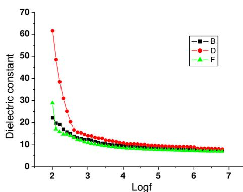
Figure (3.17): Plot of dielectric constant vs.  $\log(f)$  for (B) Sample 3.  $\text{Pb}_{0.989}\text{Fe}_{0.011}\text{C}_4\text{H}_4\text{O}_6 \cdot 1.9\text{H}_2\text{O}$  (D) sample 4.  $\text{Pb}_{0.993}\text{Fe}_{0.007}\text{C}_4\text{H}_4\text{O}_6 \cdot 0.5\text{H}_2\text{O}$  and (F) sample 5.  $\text{Pb}_{0.994}\text{Fe}_{0.006}\text{C}_4\text{H}_4\text{O}_6 \cdot 0.17\text{H}_2\text{O}$
