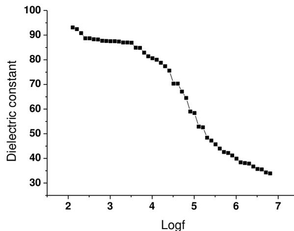
**Figure (3.15): Plot of dielectric constant vs. log(f) for pure  $\text{PbC}_4\text{H}_4\text{O}_6 \cdot 2.4\text{H}_2\text{O}$**
