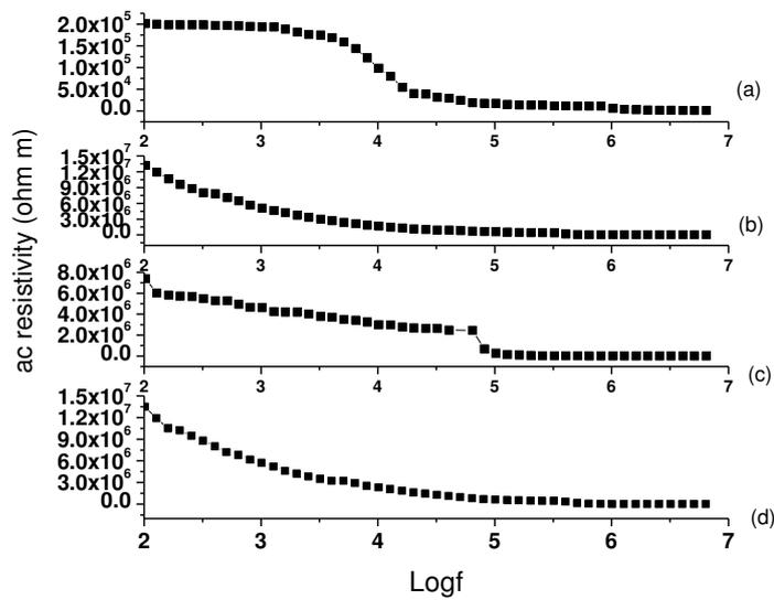
**Figure (3.20): Plot of resistivity versus log f (a)  $\text{PbC}_4\text{H}_4\text{O}_6 \cdot 2.4\text{H}_2\text{O}$  sample-1 (b)  $\text{Pb}_{0.989}\text{Fe}_{0.011}\text{C}_4\text{H}_4\text{O}_6 \cdot 1.9\text{H}_2\text{O}$  sample-3, (c)  $\text{Pb}_{0.993}\text{Fe}_{0.007}\text{C}_4\text{H}_4\text{O}_6 \cdot 0.5\text{H}_2\text{O}$  sample-4 and (d)  $\text{Pb}_{0.994}\text{Fe}_{0.006}\text{C}_4\text{H}_4\text{O}_6 \cdot 0.17\text{H}_2\text{O}$  sample-5**
