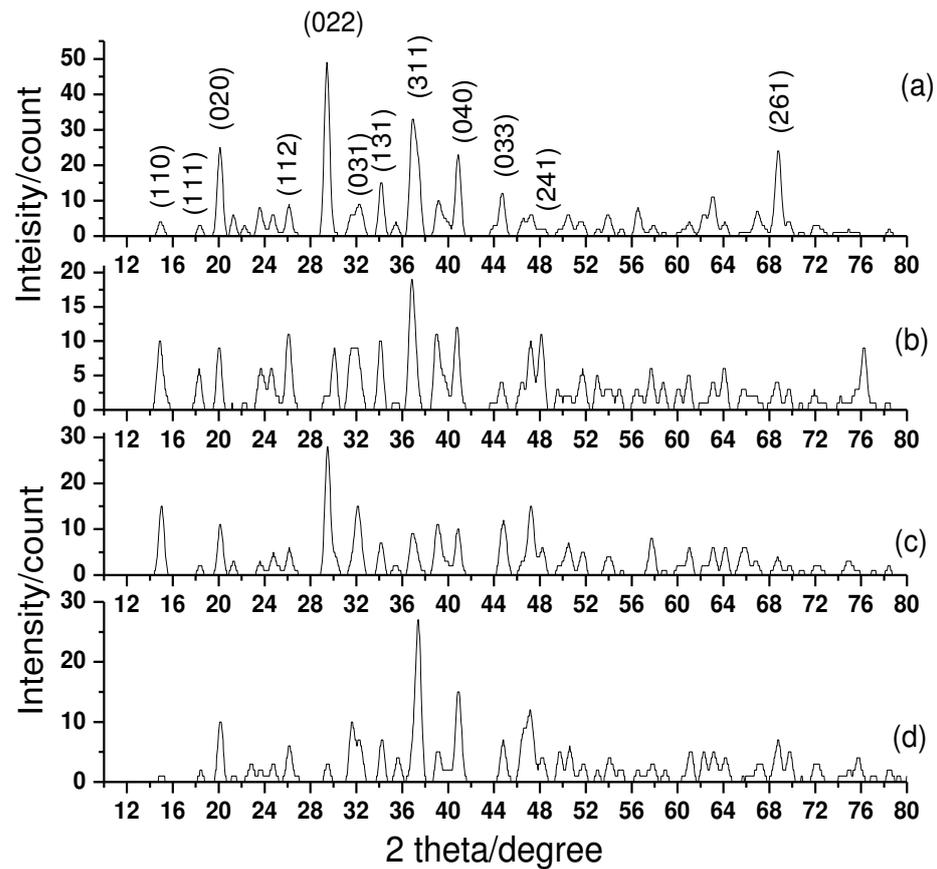
**Figure (3.3):** The powder XRD patterns for (a)  $\text{PbC}_4\text{H}_4\text{O}_6 \cdot n\text{H}_2\text{O}$
