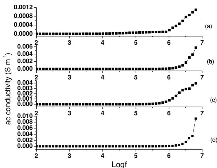
**Figure (3.19):** Plot of conductivity versus logf (a)  $\text{PbC}_4\text{H}_4\text{O}_6 \cdot 2.4\text{H}_2\text{O}$  sample-1 (b)  $\text{Pb}_{0.989}\text{Fe}_{0.011}\text{C}_4\text{H}_4\text{O}_6 \cdot 1.9\text{H}_2\text{O}$  sample-3, (c)  $\text{Pb}_{0.993}\text{Fe}_{0.007}\text{C}_4\text{H}_4\text{O}_6 \cdot 0.5\text{H}_2\text{O}$  sample-4 and (d)  $\text{Pb}_{0.994}\text{Fe}_{0.006}\text{C}_4\text{H}_4\text{O}_6 \cdot 0.17\text{H}_2\text{O}$  sample-5
