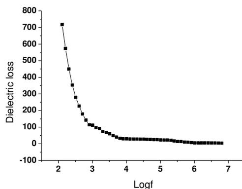
Figure (3.16): Plot of dielectric loss vs.  $\log(f)$  for pure  $\text{PbC}_4\text{H}_4\text{O}_6 \cdot 2.4\text{H}_2\text{O}$
