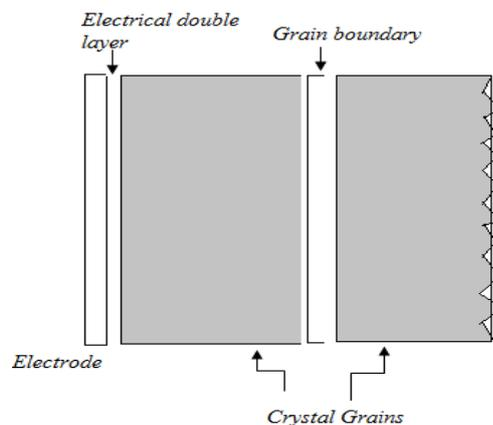
**Figure (3.10): Maxwell's model of layered dielectric**
