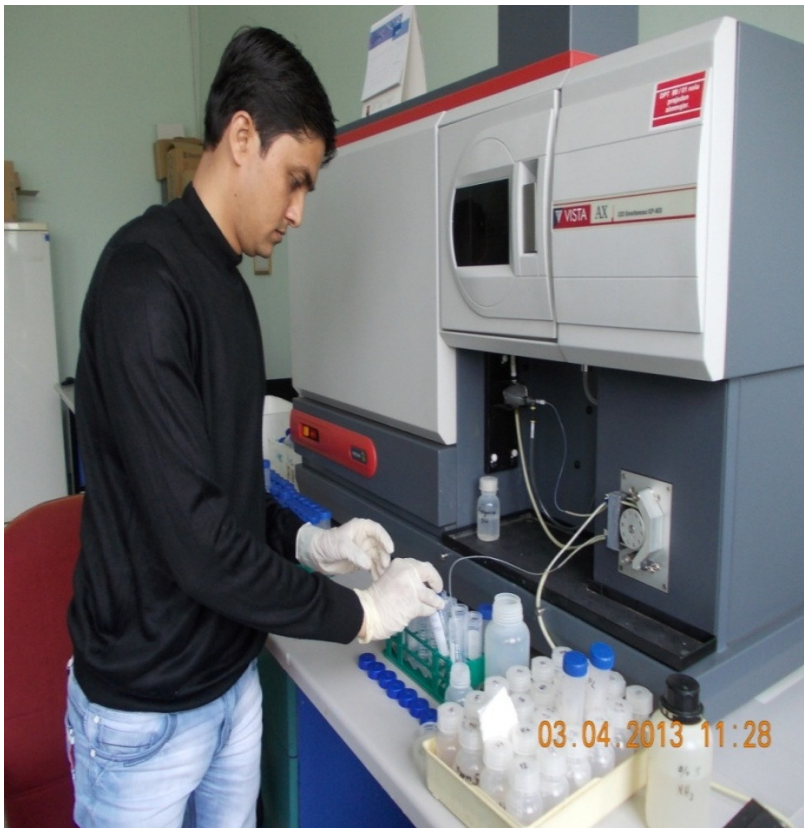
Figure 4.2: Elemental Analysis of digested wheat flour samples in ICP-AES machine at Soil Laboratory, Selcuk University, Konya, Turkey
