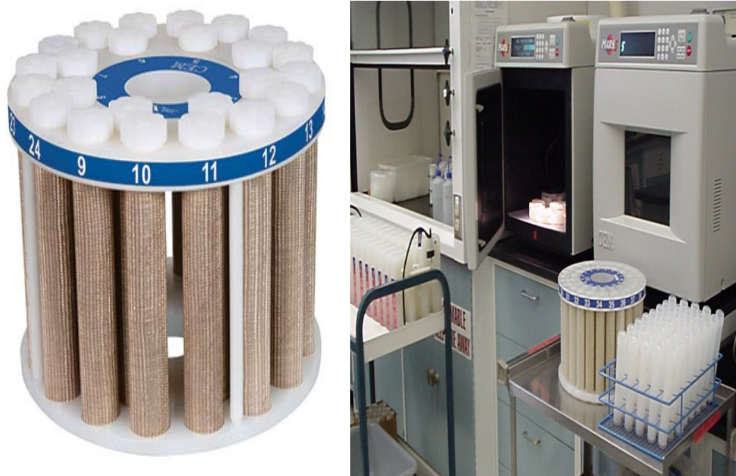
Figure 4.1: Sample Digestion Vessels and MARS-CEM Xpress Closed Microwave Digestion System
