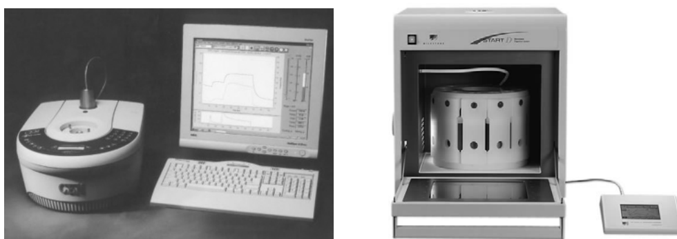
Figure 1.2: General View of Monomode CEM Discover (left) and Multimode MILESTONE Start (right) Systems
