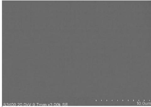
Fig. 1.4(a) SEM picture of a glass before crystallization
