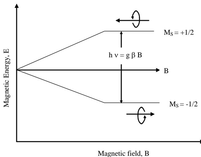
Fig. 1.10 Zeeman energy for a single unpaired electron as function of magnetic field B. A magnetic dipole aligned parallel to B has lower energy while a magnetic dipole aligned antiparallel to B has higher energy.
