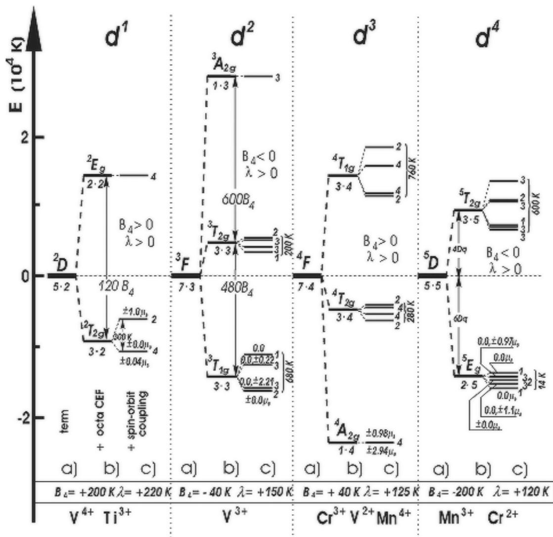
Fig. 1.8 (b) Detailed spectral information on various transition metal (from  $d^1$  to  $d^4$ ) ions.
