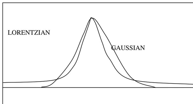
Fig. 1.11 The characteristic Lorentzian and Gaussian line shapes.
