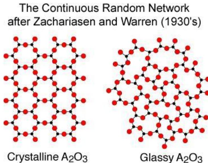
**Fig. 1.1** Two dimensional schematic of crystalline and non-crystalline (glass) materials.
