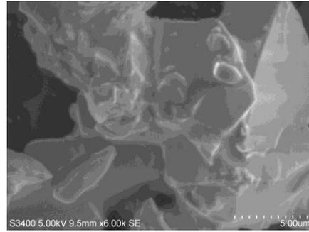
Fig. 1.4(b) SEM picture of a glass after crystallization
