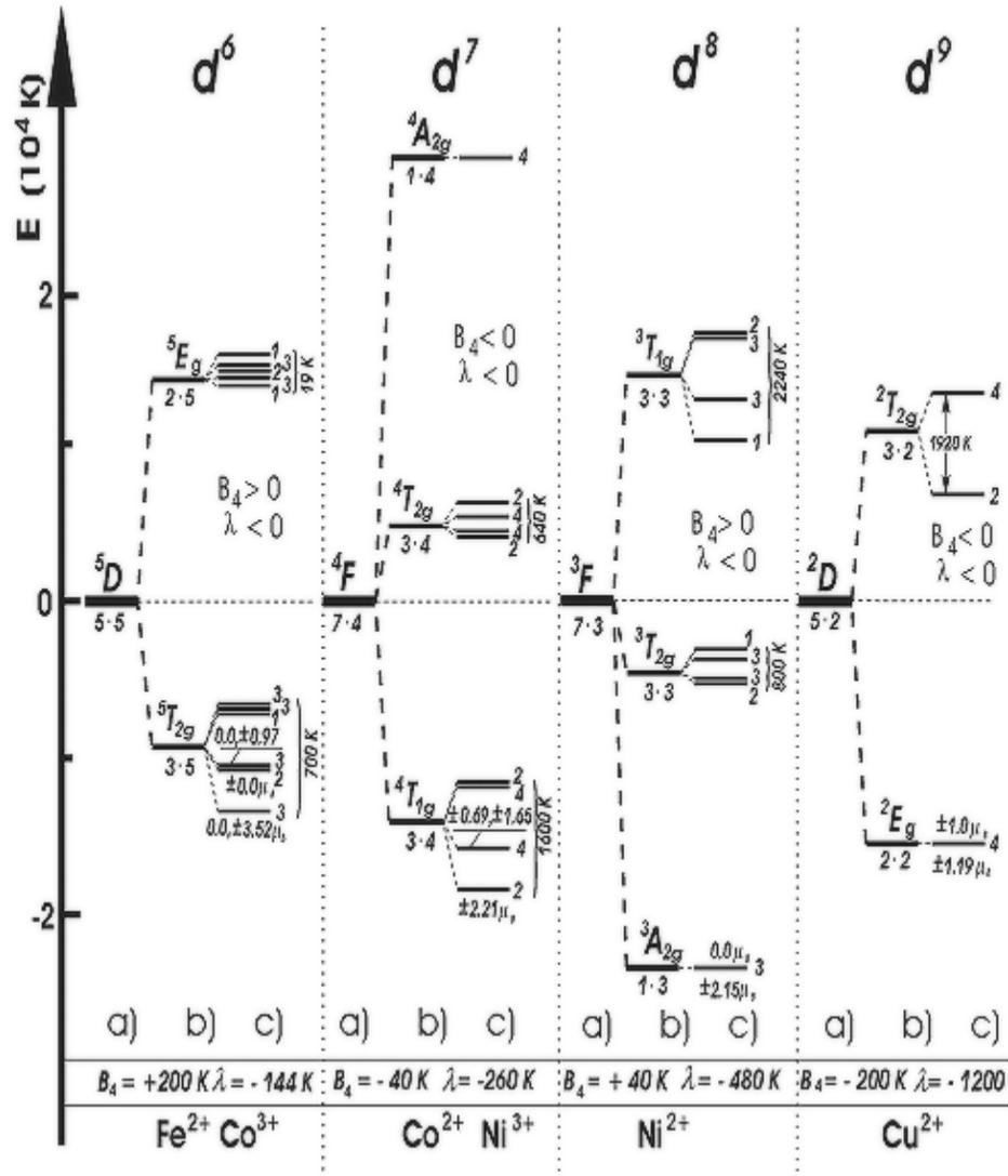
Fig. 1.8 (c) Detailed spectral information on various transition metal (from  $d^6$  to  $d^9$ ) ions
