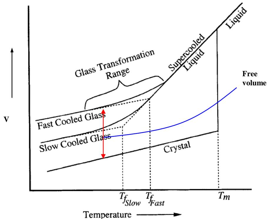
Fig. 1.3 Schematic illustration of the change in volume with temperature as super cooled liquid is cooled through the glass transition temperature  $T_g$ .
