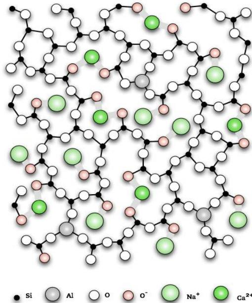
Fig. 1.2 Structure of a glass with modifier oxides
