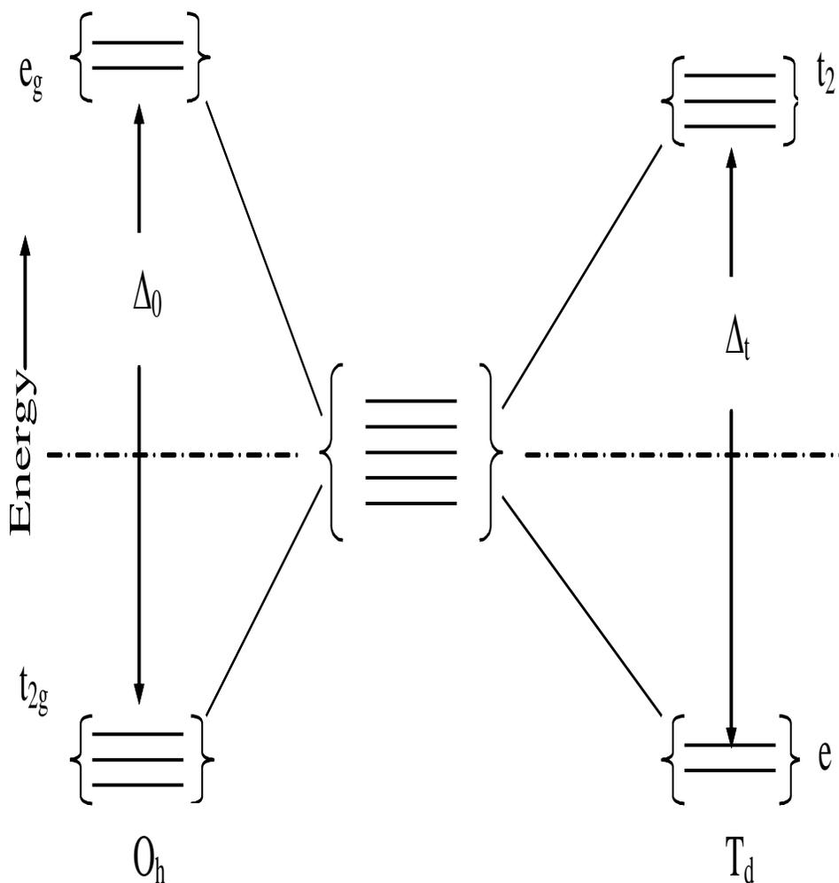
Fig. 1.9 Diagram showing relative energy of  $e_g$  and  $T_{2g}$  orbitals resulting from splitting of d orbitals by octahedral environments.
