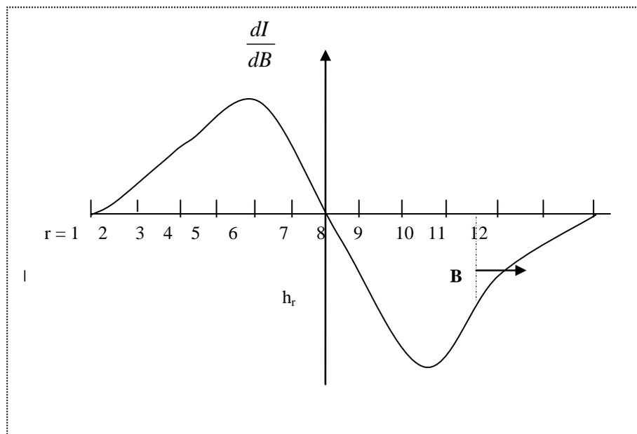
Fig. 1.12 The method of finding the area under the first derivative absorption curve by numerical double integration method.
