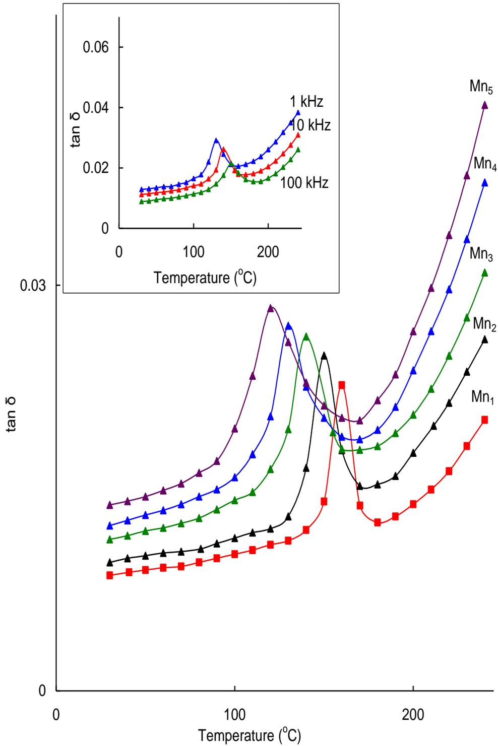
Fig.4.13 A comparison plot of variation of dielectric loss with temperature at 10 kHz for  $\text{PbO-Sb}_2\text{O}_3\text{-As}_2\text{O}_3\text{: MnO}$  glass ceramics. Inset gives the variation of dielectric loss with temperature at different frequencies of glass ceramic  $\text{Mn}_3$ .
