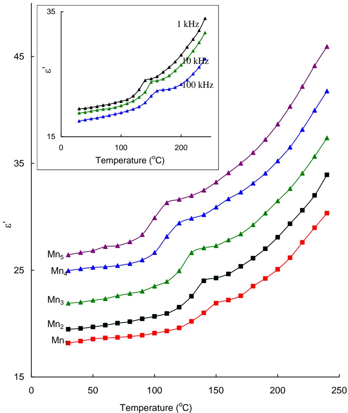
Fig. 4.12 A comparison plot of variation of dielectric constant with temperature at 1 kHz for PbO-Sb<sub>2</sub>O<sub>3</sub>-As<sub>2</sub>O<sub>3</sub>: MnO glass ceramics. Inset gives the variation of dielectric constant with temperature at different frequencies of glass ceramic Mn<sub>4</sub>.
