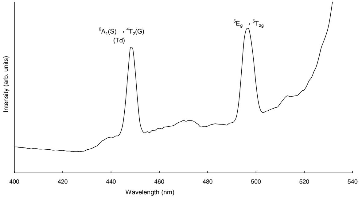
Fig. 4.7 Excitation spectrum of glass ceramic  $Mn_2$  recorded at room temperature ( $\lambda_{\text{emission}} = 550$  nm).
