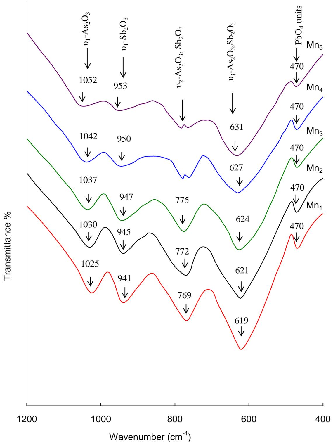
Fig. 4.10 IR spectra of PbO-Sb<sub>2</sub>O<sub>3</sub>-As<sub>2</sub>O<sub>3</sub>: MnO glass ceramics.
