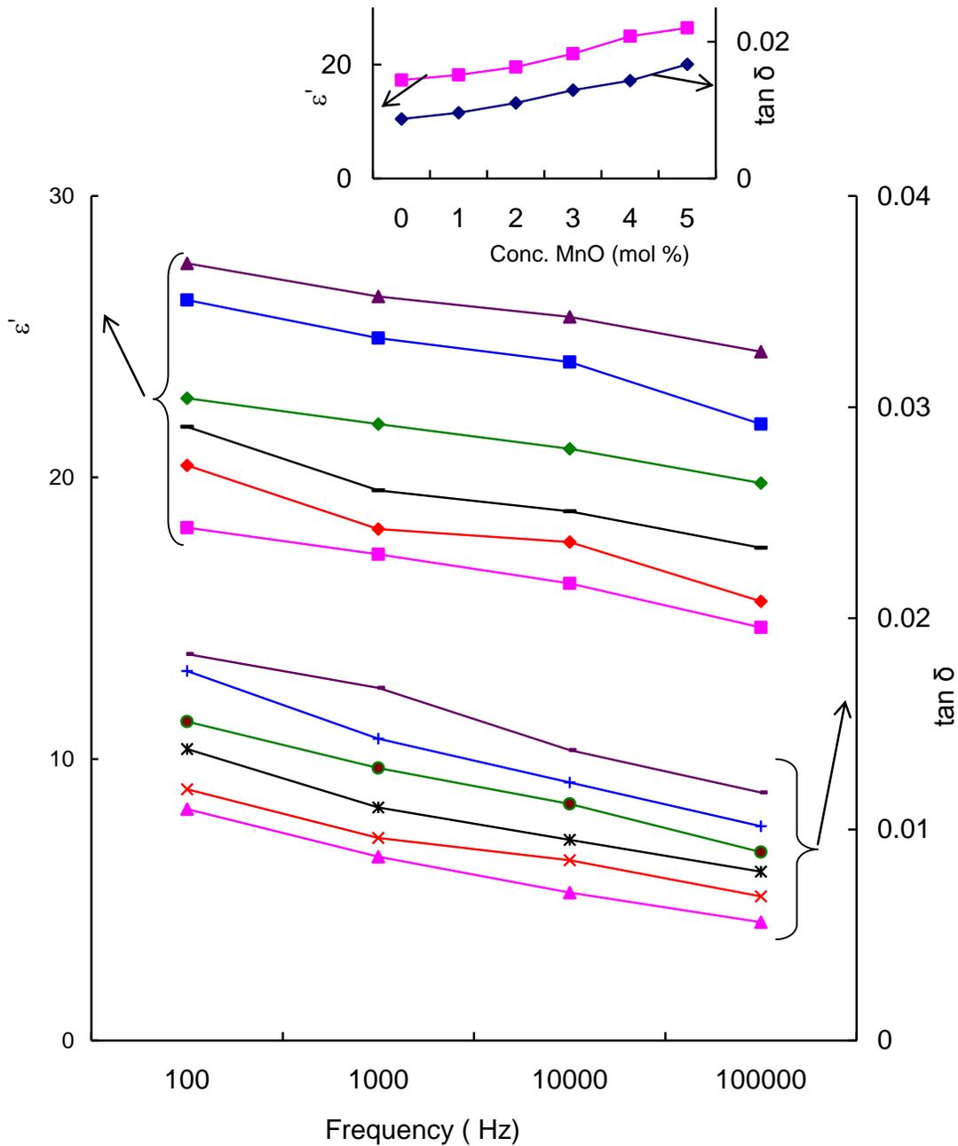
Fig. 4.11 Variation of dielectric constant and loss with frequency of PbO-Sb<sub>2</sub>O<sub>3</sub>-As<sub>2</sub>O<sub>3</sub>: MnO glass ceramics measured at room temperature. Inset represents the variation of dielectric constant and loss at room temperature with the concentration of the crystallizing agent.
