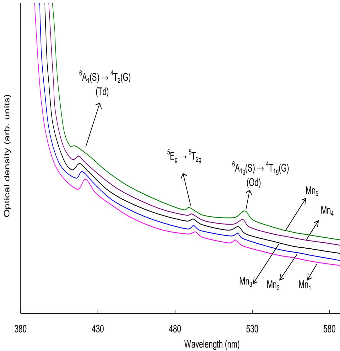
Fig. 4.5 Optical absorption spectra of PbO-Sb<sub>2</sub>O<sub>3</sub>-As<sub>2</sub>O<sub>3</sub>: MnO glass ceramics.
