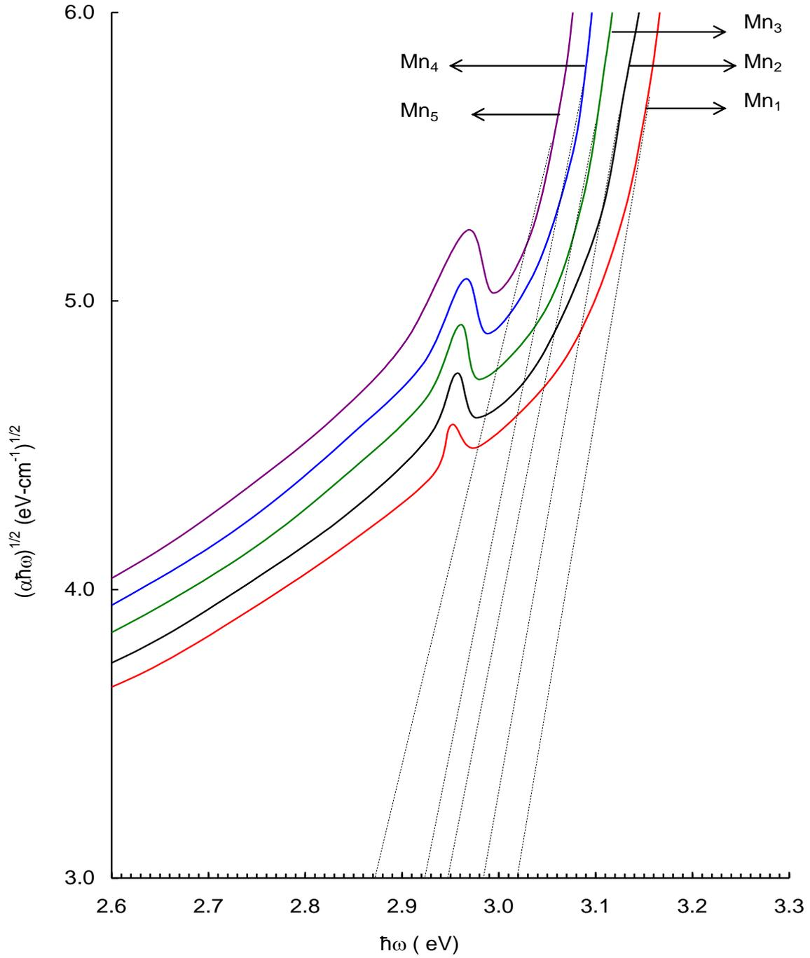
Fig. 4.6 Plots to evaluate optical band gaps for PbO-Sb<sub>2</sub>O<sub>3</sub>-As<sub>2</sub>O<sub>3</sub>:MnO glass ceramics.
