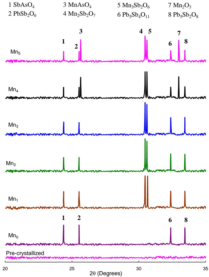
Fig. 4.3 XRD patterns of  $\text{PbO-Sb}_2\text{O}_3\text{-As}_2\text{O}_3\text{:MnO}$  glass ceramics.
