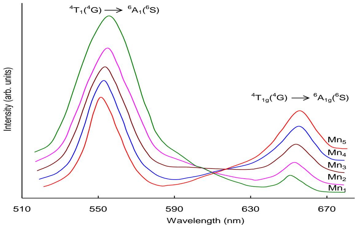
Fig. 4.8 Emission spectra of  $PbO-Sb_2O_3-As_2O_3: MnO$  glass ceramics recorded at room temperature ( $\lambda_{\text{exc}} = 449$  nm).
