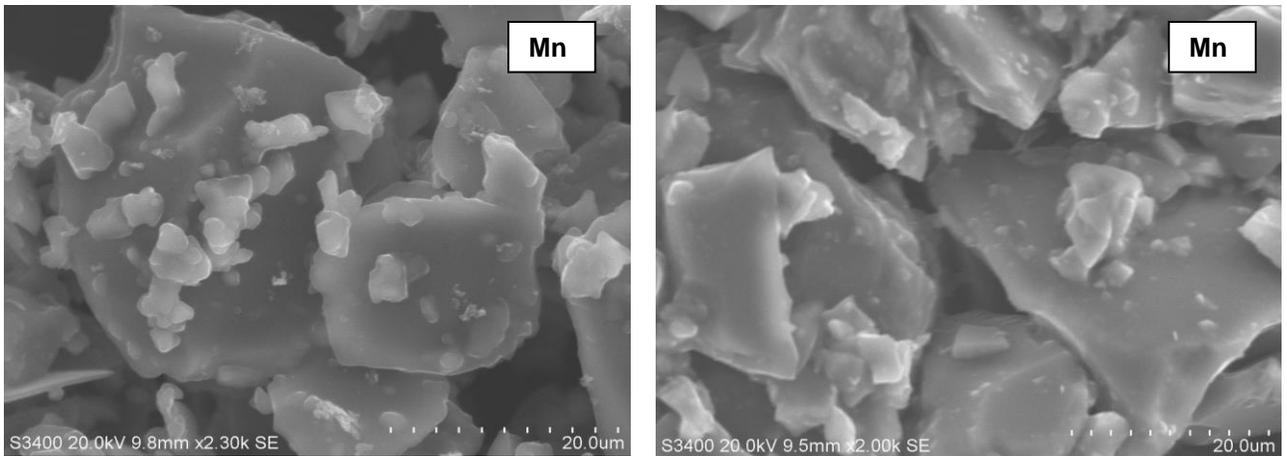
Fig 4.1 SEM images for some of the crystallized  $\text{PbO-Sb}_2\text{O}_3\text{-As}_2\text{O}_3\text{:MnO}$  glasses
