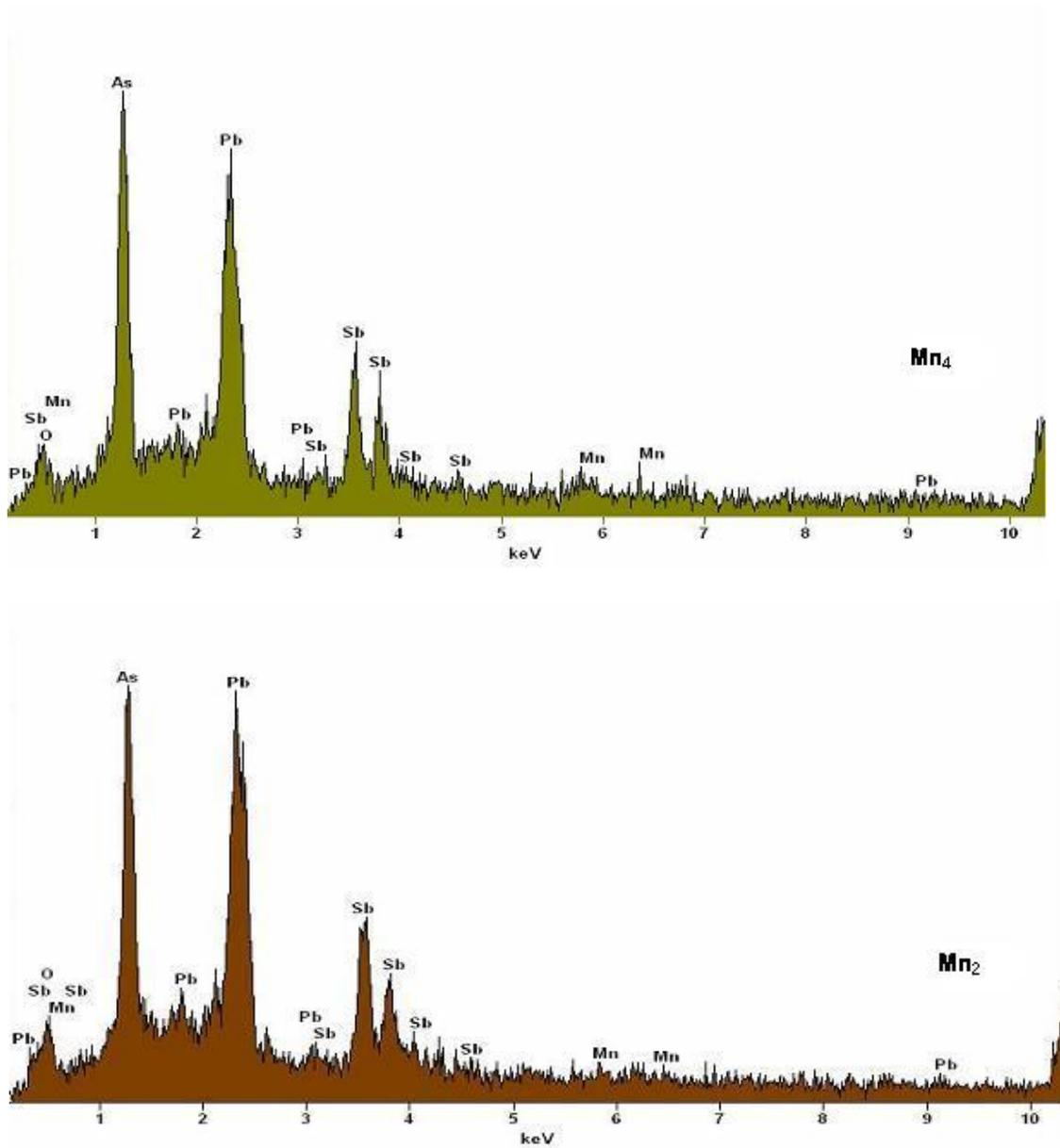
Fig 4.2 EDS spectra of some of the PbO-Sb<sub>2</sub>O<sub>3</sub>-As<sub>2</sub>O<sub>3</sub>: MnO glass ceramics.
