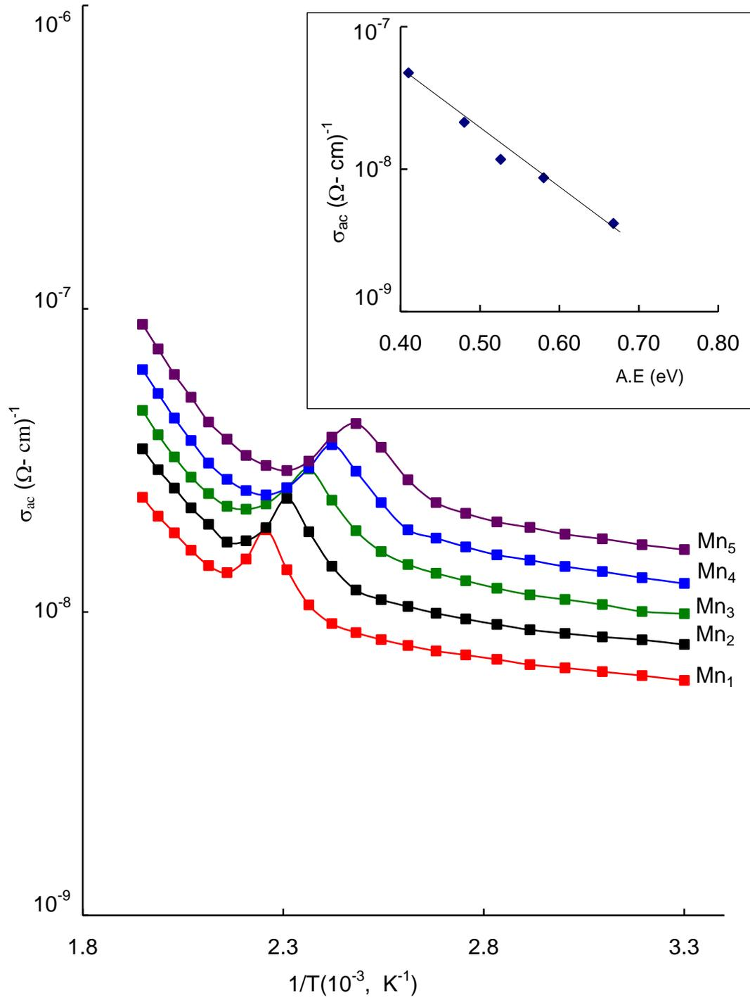
Φιγ. 4.14 ζαριατιον οφ  $\sigma_{ac}$  with  $1/T$  at 100 kHz of  $\text{PbO-Sb}_2\text{O}_3\text{-As}_2\text{O}_3$ : MnO glass ceramics. Inset represents the variation of a.c. conductivity with activation energy for conduction.
