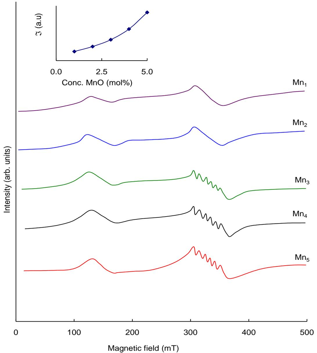
Fig. 4.9 ESR spectra of  $PbO-Sb_2O_3-As_2O_3:MnO$  glass ceramics recorded at room temperature. Inset gives the dependence of intensity factor for  $g = 2.0$  signal with conc. of MnO.
