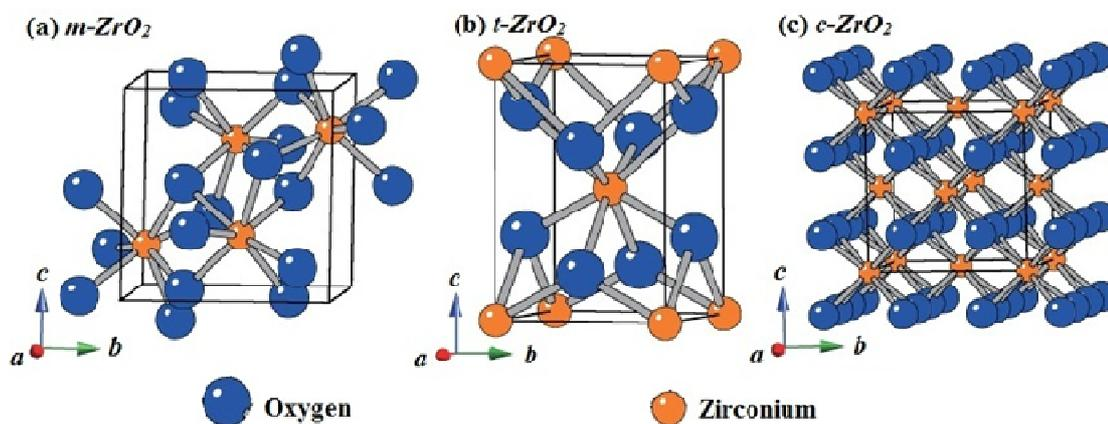
**Figure 1.4:** Crystal structures of (a) monoclinic,  $m\text{-ZrO}_2$ ; (b) tetragonal,  $t\text{-ZrO}_2$  and (c) cubic,  $c\text{-ZrO}_2$ .
