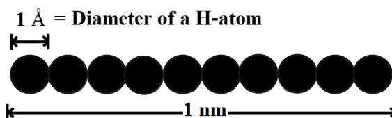
**Figure 1.1:** Length of 10 hydrogen atoms, which is equal to 1 nm.
