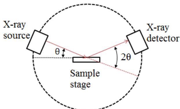
**Figure 1.6:** Schematic diagram of x-ray diffraction showing basic components.
