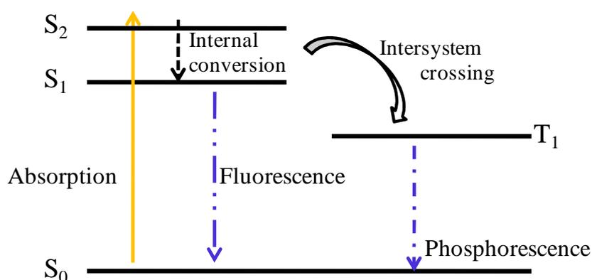
**Figure 1.2:** Jablonski diagram showing fluorescence and phosphorescence.
