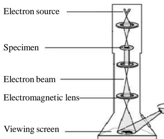
**Figure 1.7:** Schematic diagram of a TEM.
