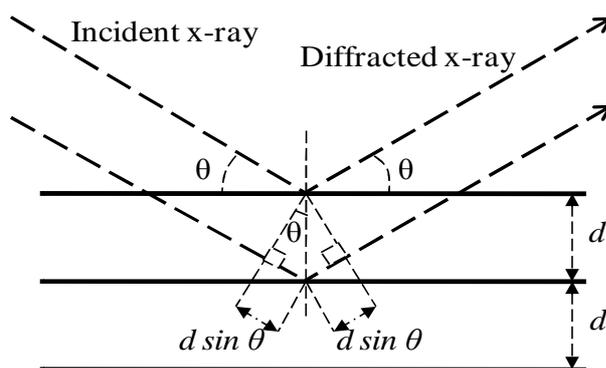
**Figure 1.5:** Schematic diagram of x-ray diffraction and Bragg's law.
