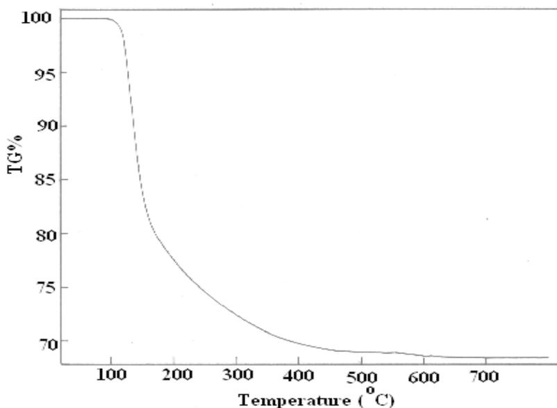
**Figure 3.13** Thermogravimetric analysis of SPB crystal
