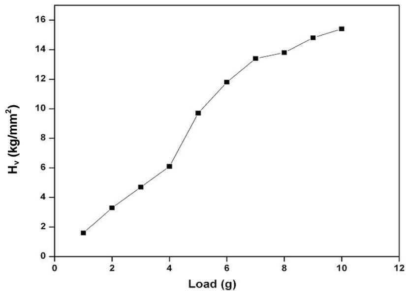
Figure 3.15 Dependence of hardness number of SPB crystal on load
