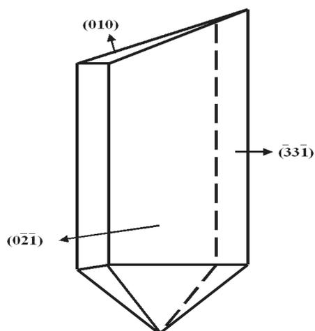
**Figure 3.3 Morphology of sodium pentaborate**
