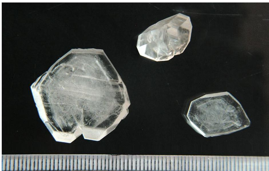
**Figure 3.2** As grown crystals of sodium pentaborate
