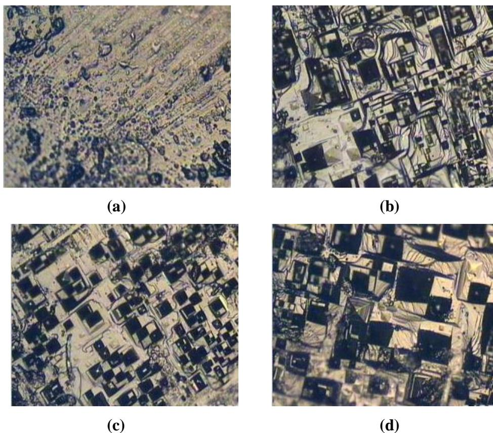
**Figure 3.8** (a) As grown surface of SPB crystal (b), (c) & (d) etched surfaces of SPB by water for 5 sec, 10 sec and 15 sec, respectively (magnification 160 X)
