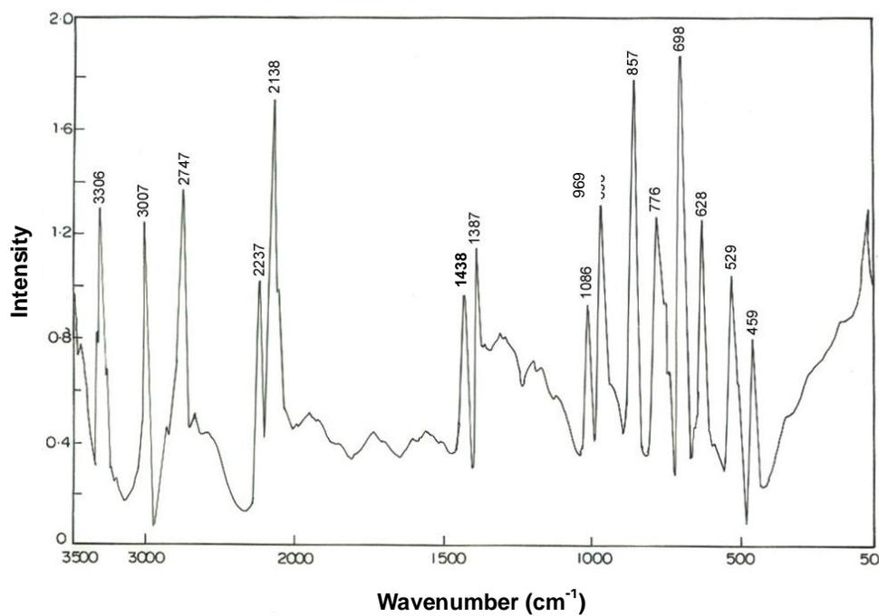
Figure 3.7 FT-Raman spectrum of SPB
