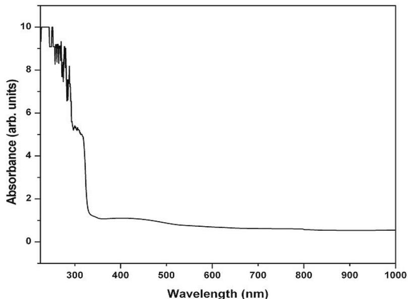
**Figure 3.12 UV-Vis. Spectrum of SPB crystal**
