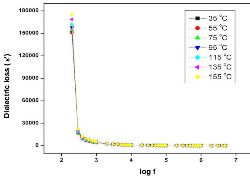
**Figure 3.10** Dependence of dielectric loss of SPB with log f
