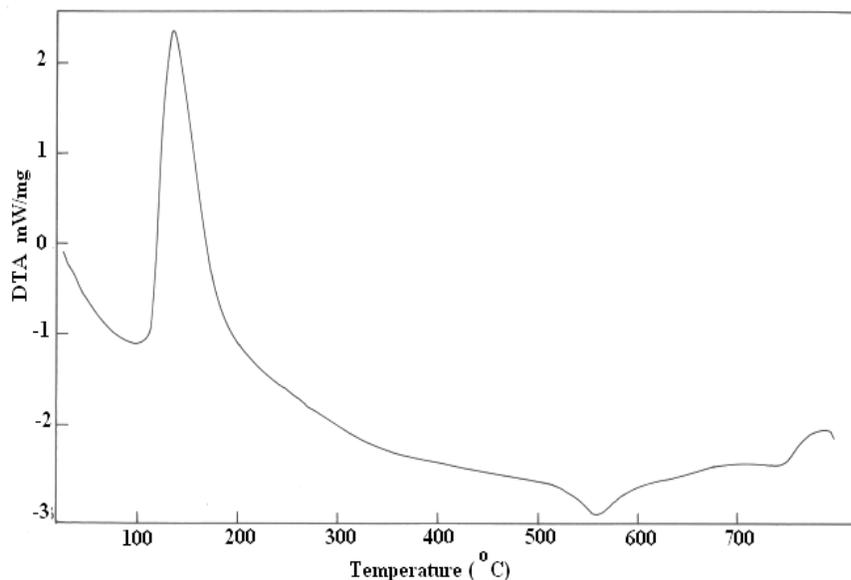
**Figure 3.14** Differential thermal analysis of SPB crystal
