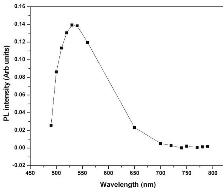
**Figure 3.5** Photoluminescence spectrum of sodium pentaborate (SPB)
