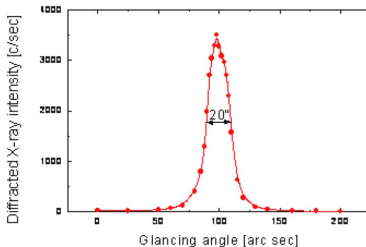
**Figure 3.4** High resolution X-ray diffraction curve of SPB single crystal
