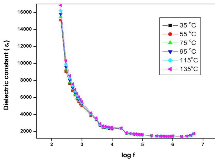
**Figure 3.9** Dependence of dielectric constant of SPB with log f
