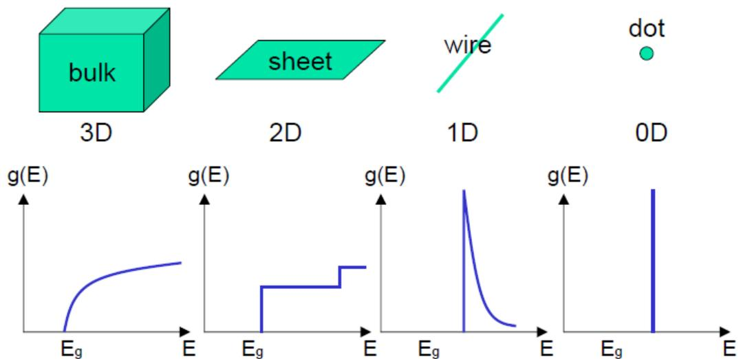
**Fig. 1.2:** Density of electron states of a semiconductor as a function of dimension. The optical absorption spectrum is roughly proportional to the density of states.
