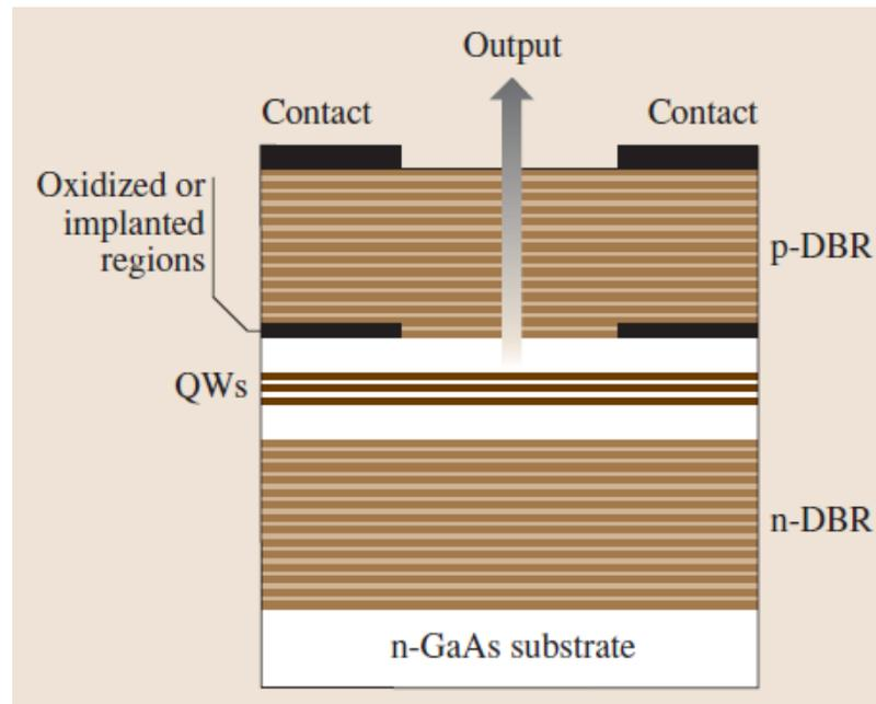
**Fig. 1.8:** Schematic diagram of a VCSEL. The QWs that comprise the gain medium are placed at the centre of the cavity formed between two distributed Bragg reflector mirrors. Oxidised or proton-implanted regions provide the lateral confinement for both the current and the optical mode.
