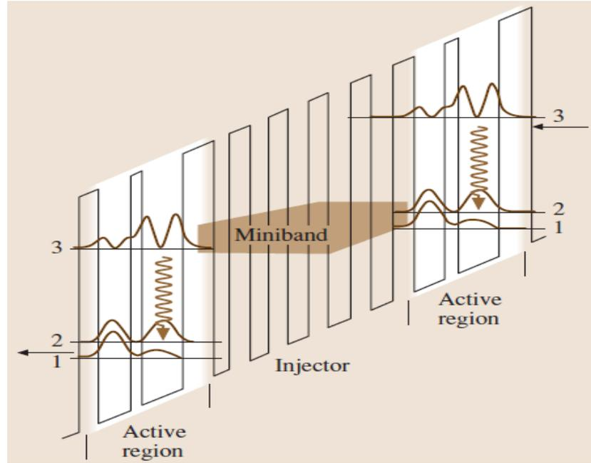
**Fig. 1.9:** Conduction band diagram for two active regions of an InGaAs/AlInAs quantum cascade laser, together with the intermediate mini-band injector region. The levels in each active region are labelled according to their quantum number  $n$ , and the corresponding wave function probability densities are indicated. Laser transitions are indicated by the wavy arrows, while electron tunnelling processes are indicated by the straight arrows.
