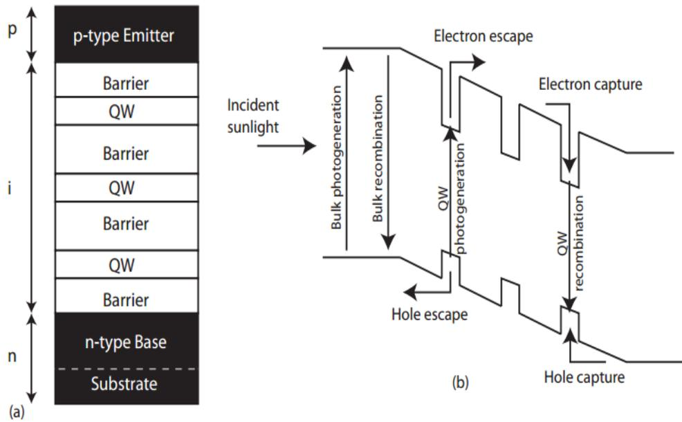
**Fig. 1.10:** (a) Quantum well p-i-n layer structure. (b) Band diagram for the quantum well p-i-n solar cell showing the photogeneration and recombination processes, together with the carrier capture and escape routes. (courtesy: (Ekins-Daukes et al. 2013)).
