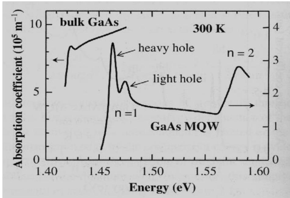
**Fig. 1.7:** Room temperature absorption spectrum of GaAs/Al<sub>0.28</sub>Ga<sub>0.72</sub>As MQW structure (Courtesy:(Han et al. 1998).
