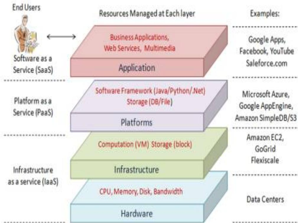
**Figure 1.6 Layered Architecture of Cloud Services [22]**
