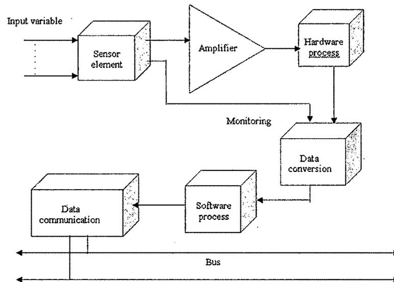
Fig 1.2: Elements of a traditional sensor
