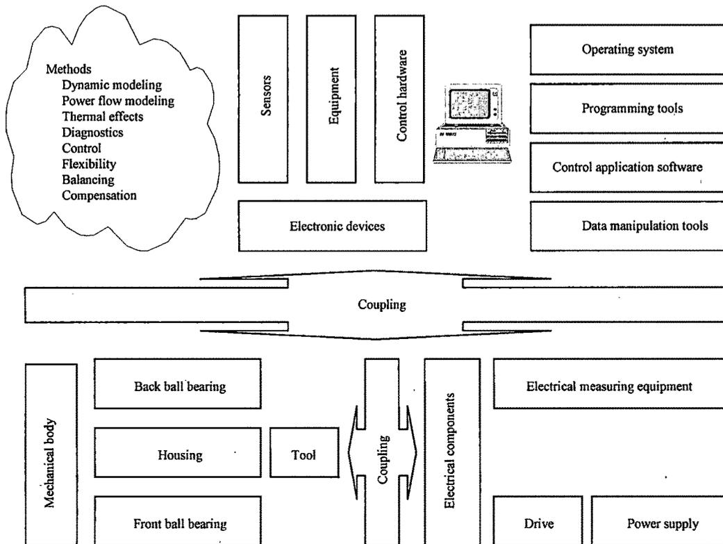
Fig. 1.1: A typical example of mechatronic system: Spindle system
