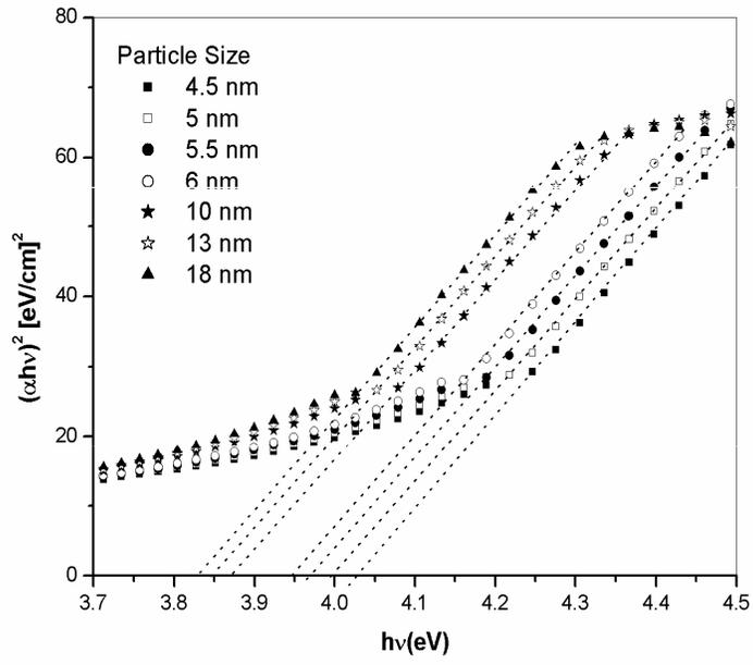
Figure 2.6 : Optical bandgap of ZnO colloids
