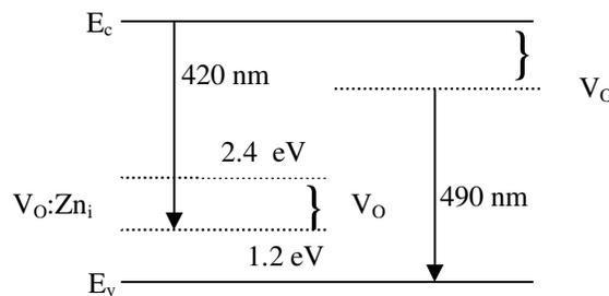
Figure 2.20: Representation of various defect levels in ZnO
