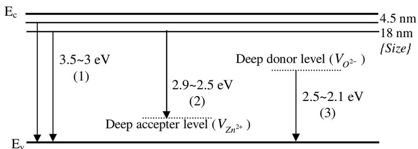
Figure 2.22: The UV and visible photoluminescence mechanism of ZnO:
